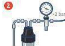
2 Check water filter (valve) and water pressure incoming water > 2 bar.
