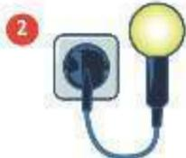
2 Use a light or appliance that there is power to the outlet. If not check the fuse box.
