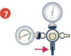
7 Check whether the ball valve of the carbon dioxide is open.
