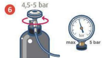
6 Make sure the CO<sub>2</sub> cylinder is open and the pressure is 3.5 to 5 bar.
