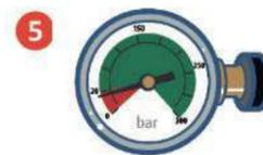
5 Check the contents of the CO<sub>2</sub> cylinder. Pressure gauge in red? Replace cylinder.
