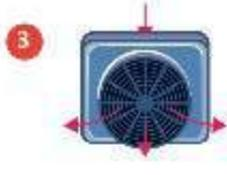
3 Check that nothing is blocking the ventilation around the cooling unit. Remove any obstructions.
